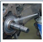
**4.** Use a cleaning agent to remove even the finest remnants of brake dust and metal particles.
