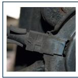
**2.** If it is not possible to remove the ABS sensor, make sure that the sensor is kept free from dirt and foreign objects.
