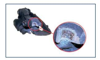
In this example, the guide/mounting for the handbrake cable on the brake caliper housing has been destroyed.
