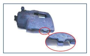
In this example, part of the brake caliper housing has been broken off and cannot be reconditioned.
