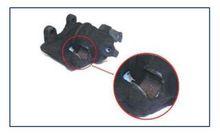
In this example, part of the brake caliper housing has been destroyed in the area of the guide sleeve.
