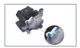
In this example, the guide sleeve housing has been destroyed.
