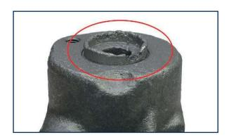
The inner cylindrical part has been corroded and is broken
