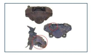
Examples of severe corrosion/rust damage on the entire housing, i.e. on the pin holes or surfaces for the brake pads.
