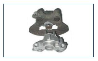
In this example, the brake caliper is incomplete and parts of the frame are missing.
