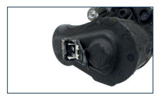
Damage or defects on the plug connector or motor for the electric hand brake.
