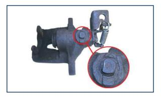
In this example, a bolt has been used. The thread is defective and toolmarks are visible.
