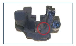
In this example, the sliding surface for the brake pads has been destroyed.
