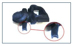
In this example, the guide for the handbrake cable has broken off.
