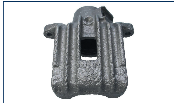
Severe corrosion/rust damage on the entire housing. The corrosion/rust damage must not be so severe that the surfaces have virtually eroded away and can no longer be reconditioned.
