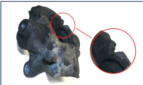
In this example, the opening for the fixing pin has been broken off/destroyed.
