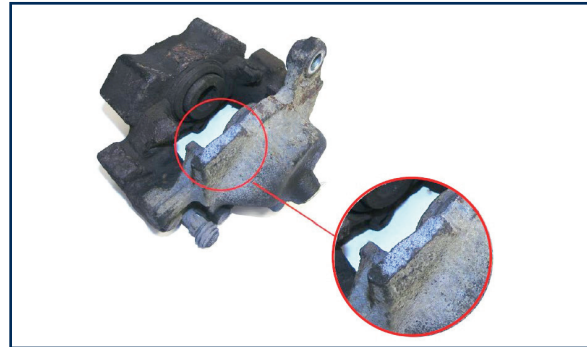
In this example, the guide sleeve housing has been destroyed.
