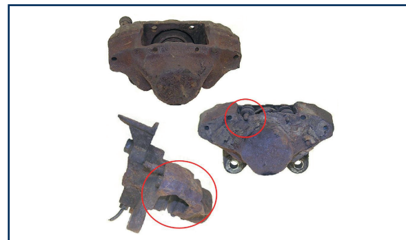
Examples of severe corrosion/rust damage on the entire housing, i.e. on the pin holes or surfaces for the brake pads. The corrosion/rust damage must not be so severe that the surfaces have virtually eroded away and can no longer be reconditioned.
