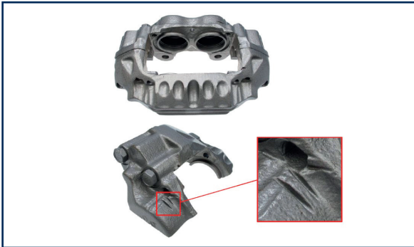
In this example, saw marks are visible on the brake caliper housing.
