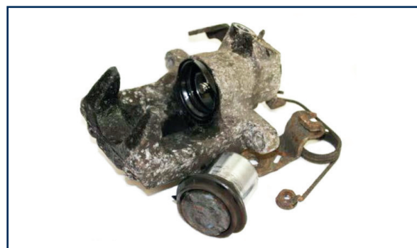
In this example, the brake caliper is incomplete and parts of the frame are missing.
