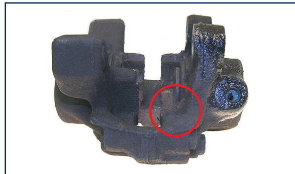
In this example, the sliding surface for the brake pads has been destroyed.
