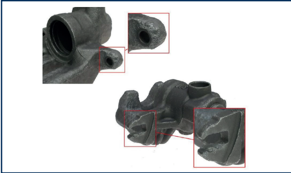
Corrosion damage on the surface of the connection for the guide pin.
