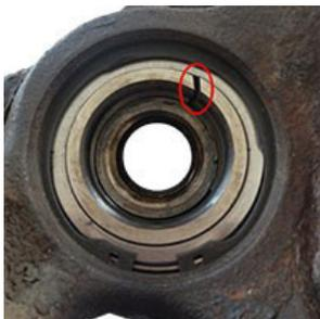
This damage is caused by the oval distortion of the wheel hub, which leads to greater pressure being applied to the bearing inner ring (see photo on the left). As a result, a precise fit can no longer be guaranteed when pressing in the wheel bearing. This generates pressure spikes that may eventually break the wheel bearing (see photo on the right).
